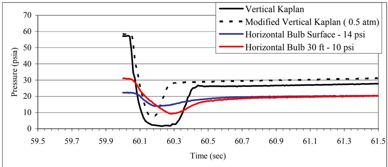
**Figure 2.3.** Comparison of the expected pressure nadirs during passage through a typical vertical Kaplan turbine, a modified vertical Kaplan turbine, and two horizontal bulb turbine passage scenarios.
