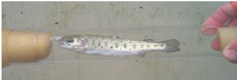
Figure 3.8. Transfer cartridge used to capture test fish before being subjected to the shear environment.
