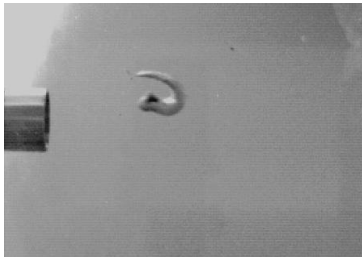
Figure 4.21. Digitized image of rainbow trout illustrating opercular flare upon exiting the nozzle during a fast-fish-to-slow-water test.
