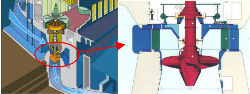
**Figure 1:** A cross section of a Kaplan turbine showing the entire turbine and its water passages on the left and details of the stay vanes, wicket gates and runner with hub and nearby water passages on the right. The water enters through the semi-spiral case, passes through the stay vanes and wicket gates, then through the runner, and finally into the draft tube, exiting to the tail waters.
