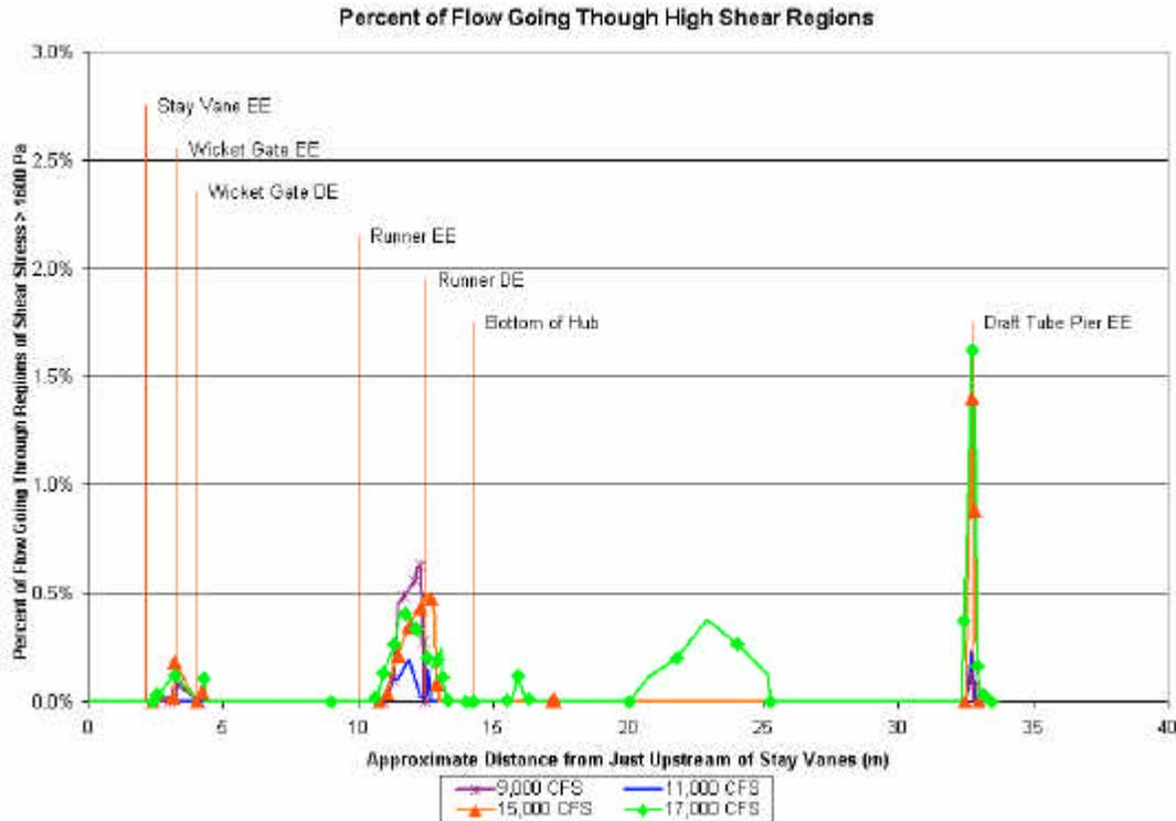
**Figure 12:** Comparison of operating conditions starting just upstream of the stay vanes. EE stands for Entrance Edge and DE is Discharge Edge. This is similar to the area ratios in figure 11, with the percentage values somewhat lower.
