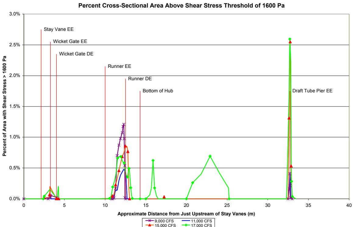
**Figure 11:** Comparison of operating conditions starting just upstream of the stay vanes. EE stands for Entrance Edge and DE is Discharge Edge. At the higher flow rates, the peak area of high shear (2.5%) occurs at the nose of one of the piers. For the runner region, the worst operating condition for shear is at low flow, 9000 cfs. This includes the shear stress within the boundary layer. All stay vanes, wicket gates, and runner blades are included in the graph.
