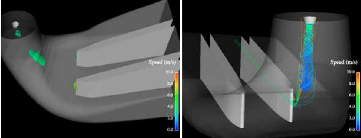
**Figure 9:** Areas of shear above 1600 Pa in the draft tube region (left). The high shear areas are represented by isoSurfaces of shear stress = 1600 Pa and are colored with speed. Streamlines showing the “torch” vortex under the hub which causes the high shear in the upstream portion of the draft tube (right). Streamlines also illustrate the poor incidence angle at the pier due to the torch vortex and uneven flow from the runner.
