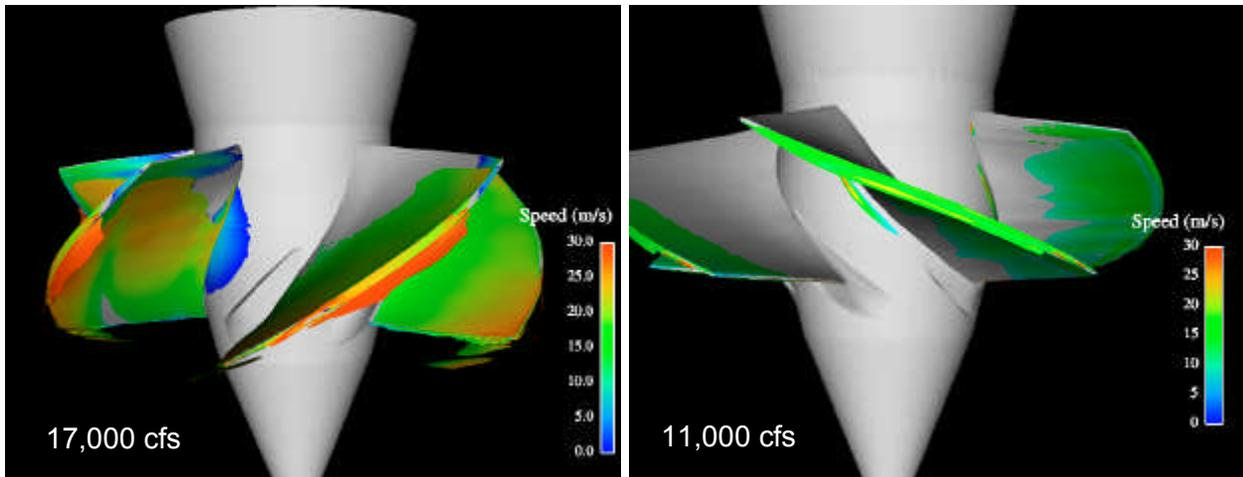
**Figure 7:** Areas in the runner region with shear stress above the fish-injury threshold of 1600 Pa at 17,000 cfs (left), and 11,000 cfs (right). The high shear areas are represented by isoSurfaces of shear stress = 1600 Pa and are colored with speed. Any non-gray area is above the threshold.
