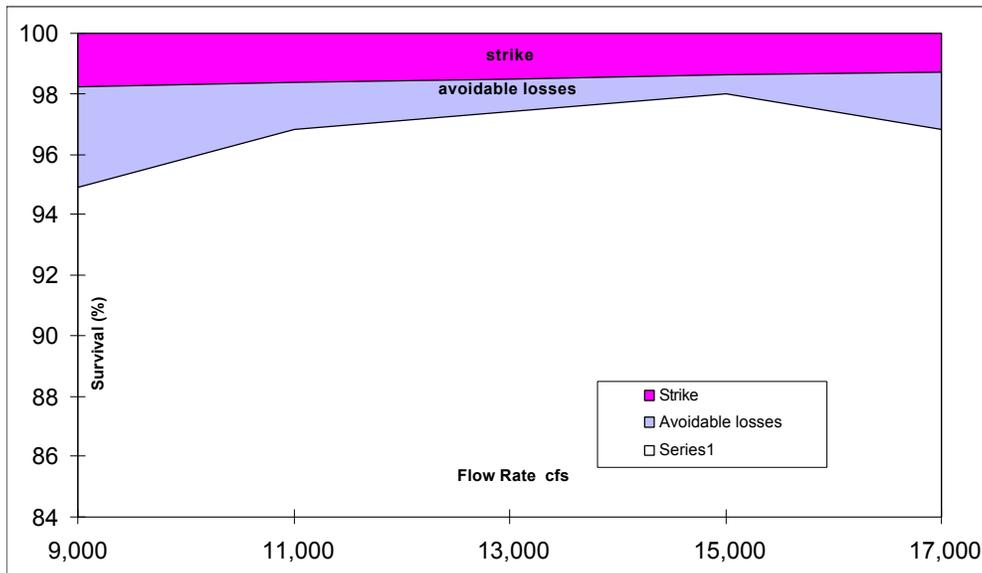
**Figure 13:** Estimates of survival for fish released near the centerline of the unit with estimated causes of mortality (Ref. 1). It is assumed that the fish passed near the center of the blade, thus avoiding any gap-related injuries and any draft tube vortex-related injuries.
