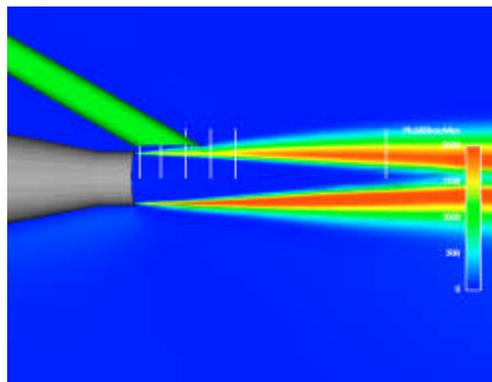
**Figure 4:**  $z/d$  (distance away from the nozzle exit divided by the diameter of the nozzle exit) for the CFD data comparison shown in figures 3 and 5. The white line closest to the nozzle exit is the  $z/d=0.079$  position and the line farthest from the nozzle exit is the  $z/d=5$  position (5 nozzle diameters downstream of the nozzle exit).
