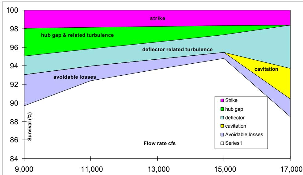
**Figure 14:** Estimates of survival for fish released near the hub with estimated causes of mortality (Ref. 1). It is assumed that the fish passed near the hub and were subject to any harmful effects of the hub gap as well as those from the draft tube vortex.
