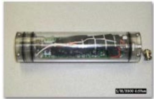
*Sensor fish prototype device.*
